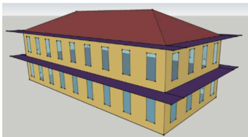
Figure-2. Colonial Office model with width of 1.80m sun shading and wall openings of 20%.
