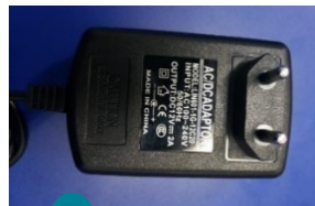
7 Figure 5. AC/DC Adapter 12V 2A
