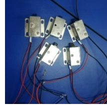
Figure 3. Solenoid Doorlock 12V 0.35A
