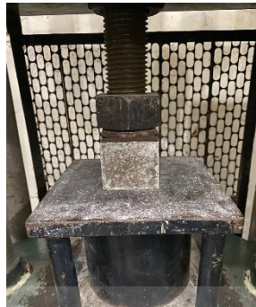
Gambar G.3 Peletakan Benda Uji Dimesin ( Compression Testing Machine )
