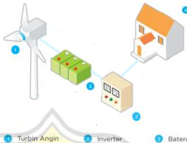
Gambar 24 – Skema Sistem Off-Grid
