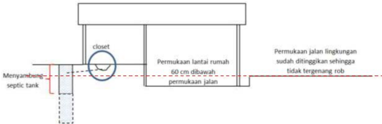
Figure-9: the solution scheme of raising the sanitation of bathroom/ toilet Source: Mulyani TH, Semarang, 2017
