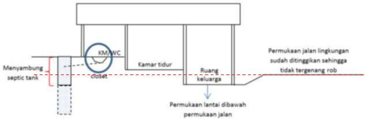
Figure-11: the solution scheme of raising the sanitation of bathroom/ toilet Source: Mulyani TH, Semarang, 2017
