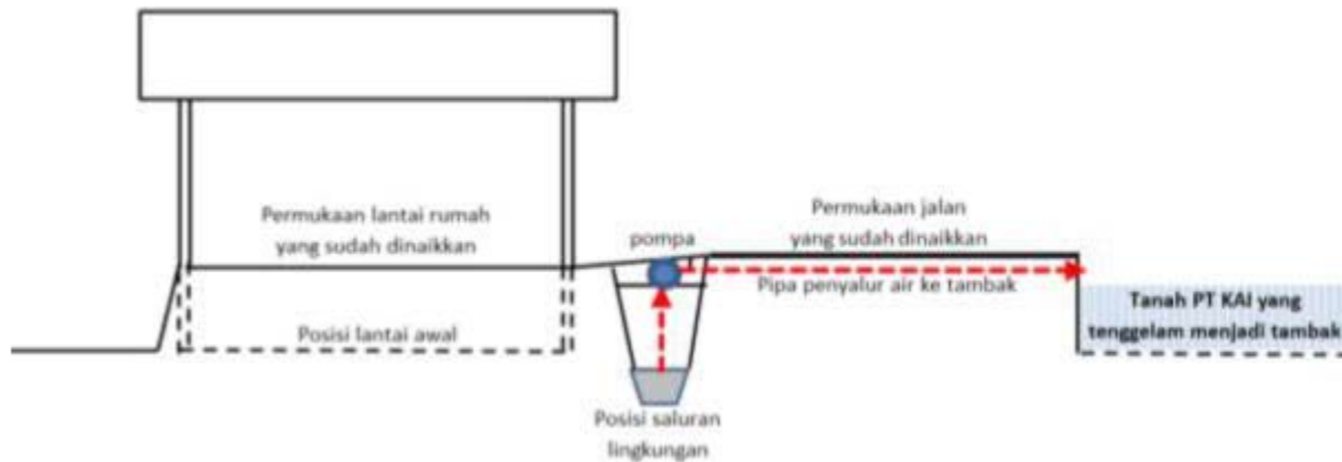
Figure-7: the scheme of the positions of environmental channel, pump, and retention pool in RW-IV of Kemijen Source: Mulyani TH, Semarang 2017
