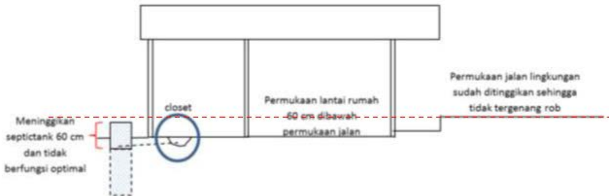
Figure-10: the solution scheme of raising the septic tank Source: Mulyani TH, Semarang, 2017
