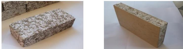
Gambar 1. Bata *Pulpy Granule – Tapioca Perva – GRC Sandwich Wall Panel*
