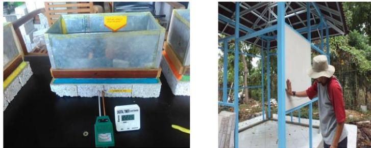
Gambar 3. Uji kedap air *Perva – GRC Sandwich Wall Panel*
