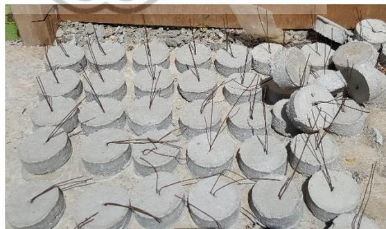
Gambar 3.86 Tahu Beton (Beton *Decking*)
