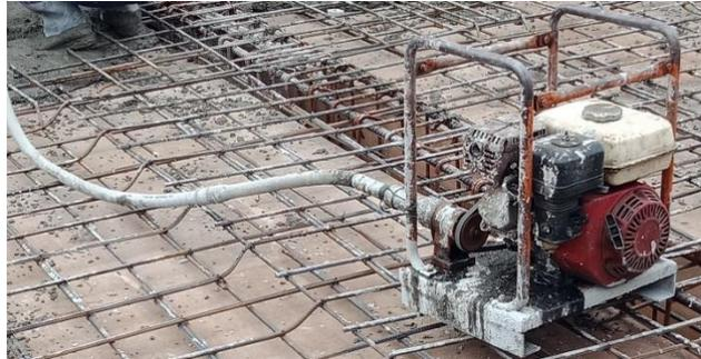
Gambar 3.81 Alat *Concrete Vibrator*
