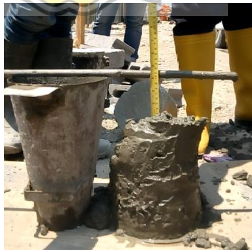
Gambar 4.2 Uji Slump Test
