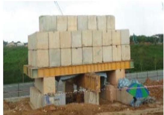
Gambar 3.11 Contoh *Loading Test*
