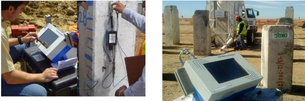
Gambar 3.18 Contoh *Pile Dynamic Analyzer* (PDA)
