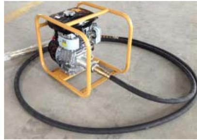
Gambar 3.66 *Concrete Vibrator*
