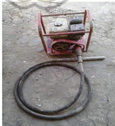
**Gambar 3.53** Mesin *Concrete Vibrator*
