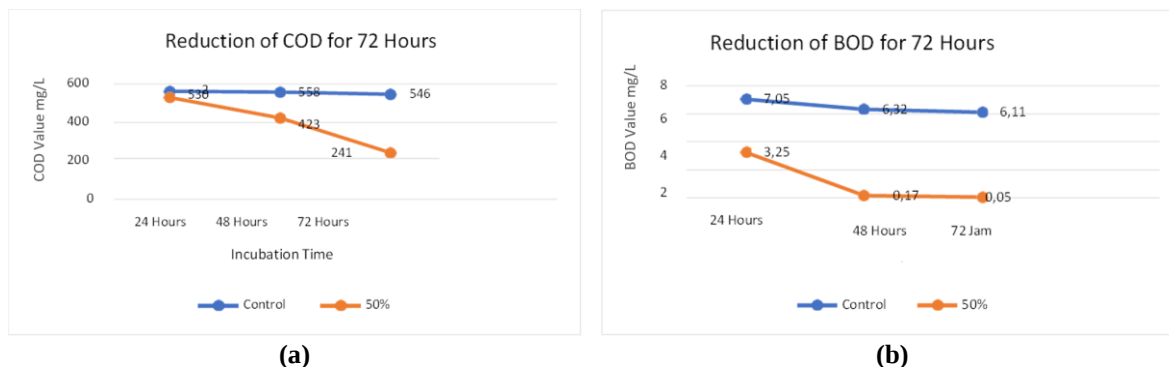
Figure 2. 50% Waste (a) COD; (b) BOD value measurement chart for 72 hours.
