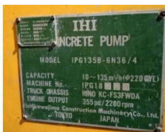
Gambar 4.9 Spesifikasi Concrete Pump Truck
