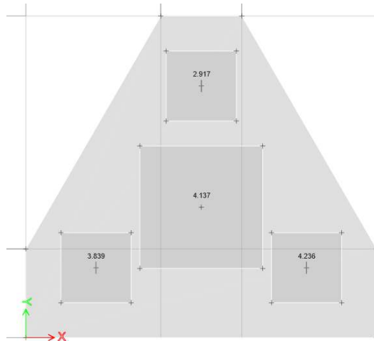
Gambar 4.3. Punching Shear pad Pile Cap
