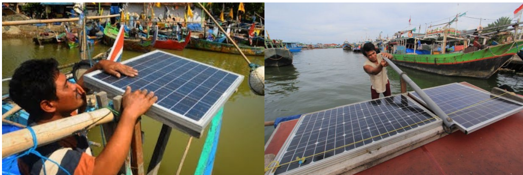
Picture 05. Local Fishermen in Karmunjawa use small PV panels on their fishing boats (Source: Antara)
