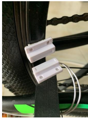
Figure 4.6 Magnetic Sensor Installed on the Bicycle
