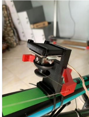
Figure 4.7 Analog Joystick Module Installed
