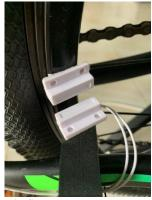
Figure 4.6 Magnetic Sensor Installed on the Bicycle
