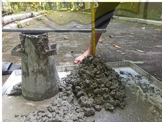
Gambar 4.4. Slump Test Beton Normal
