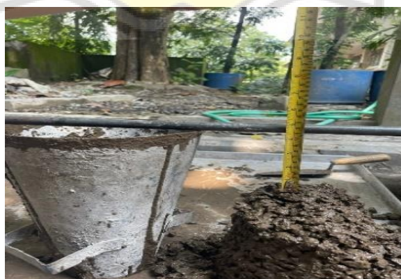
Gambar 4.3 Uji Slump Beton Normal
