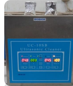
Ultrasound Extraction 37.5 min; 50°C; 45 kHz
