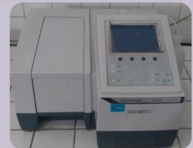
UV-Vis Spectrophotometer for DPPH assay (517 nm)
