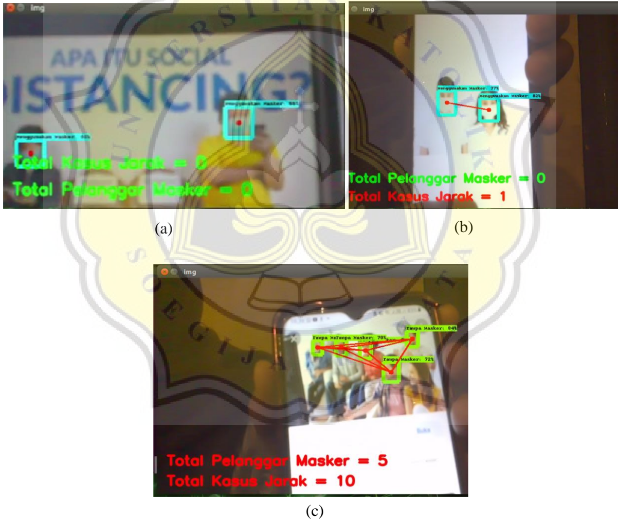
Figure 5.6 Detection Using Images (a) No Violator (b) With Violators (c) With Violators but One is Undetected
