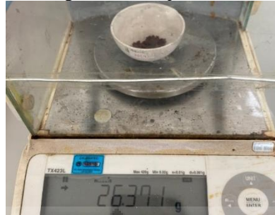
Lampiran 75. Penimbangan Sampel Hasil Uji Kadar Air
