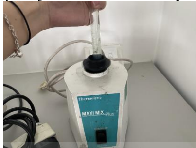
Lampiran 83. Vortex Sampel Uji Kadar Protein Lowry
