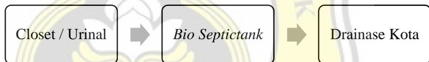
Gambar 62. Diagram Air Kotor Black Water
