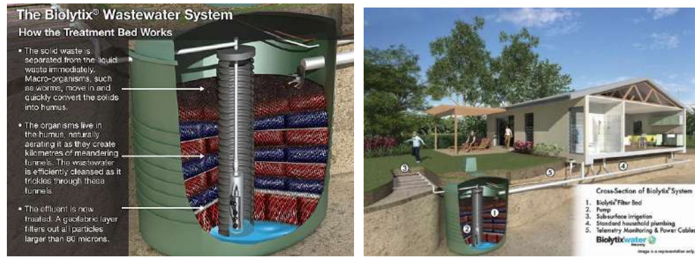
Gambar 237. Potongan skema tangki Biopod (sumber: http://www.kerryflanaganwastewater.com.au/biolytix-nz.html )
