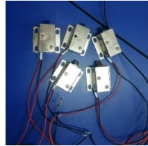
Figure 3. Solenoid Doorlock 12V 0.35A
