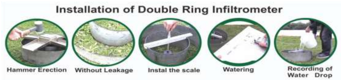
Figure 2: Instalation of Double Ring Infiltrpmetr
