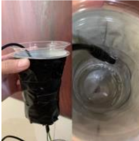
Illustration 5.2.2 TDS and LDR sensor
