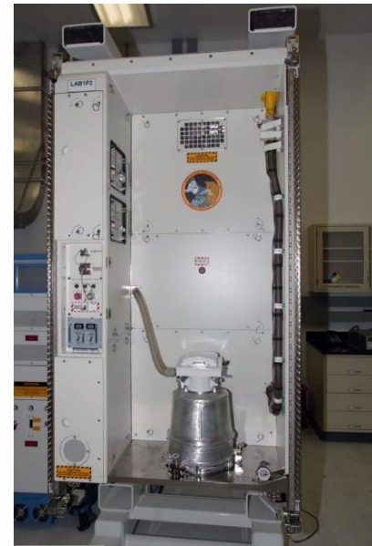
Gambar 41 Modul WHC Misi STS-126 Sumber: This photo shows the waste and hygiene compartment that will be delivered to the International Space Station on the STS-126 mission. — Google Arts & Culture
