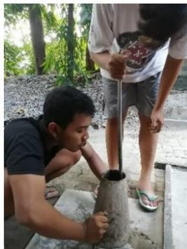
Gambar 3.8 Uji *Slump Test*
