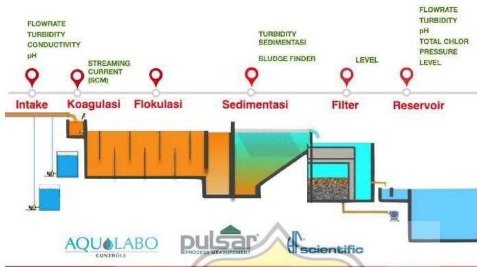
Gambar 8.8 Perencanaan Water Treatment Plant
