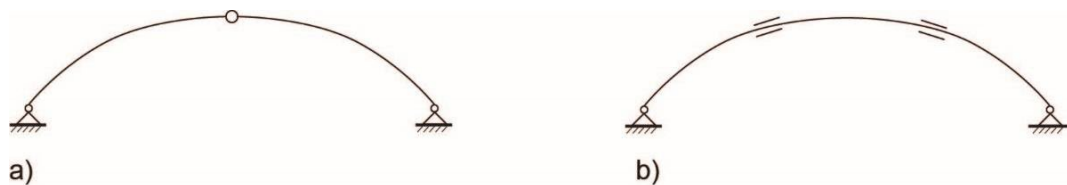
Picture 7.6 Suitable placing of joints in arch structures Source : Large-Span Timber Structure
