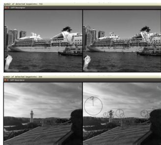
Figure 2. Keypoints from a cruiser ship image (top), and keypoints from a lighthouse image (bottom)
