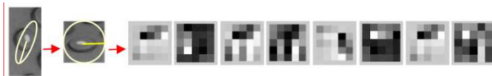
Figure 1. (from left to right) An example of Harris affine region, normalized region, and 8 maps of gradient magnitude describing SIFT descriptor [2]
