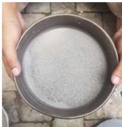
**Gambar 4.26** Proses saringan pasir
