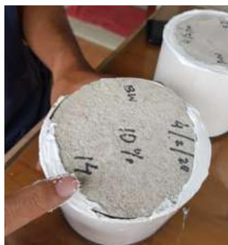
**Gambar 4.59** PVC 10 cm ditutup mortar
