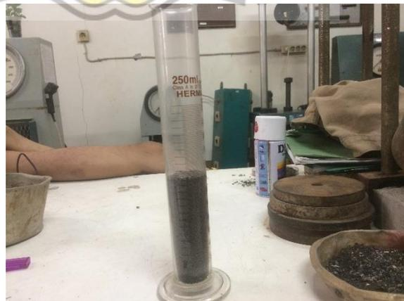
Gambar 4.10 Gelas Ukur Berisi Agregat Halus
