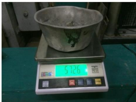
Gambar 4.24 Menimbang Wadah Berisi Agregat Kasar Kering
