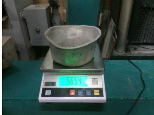
Gambar 4.21 Menimbang Wadah Berisi Agregat Halus Kering
