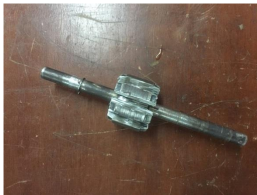
Gambar-3.1. Konstruksi rotor motor Switched Reluctance
