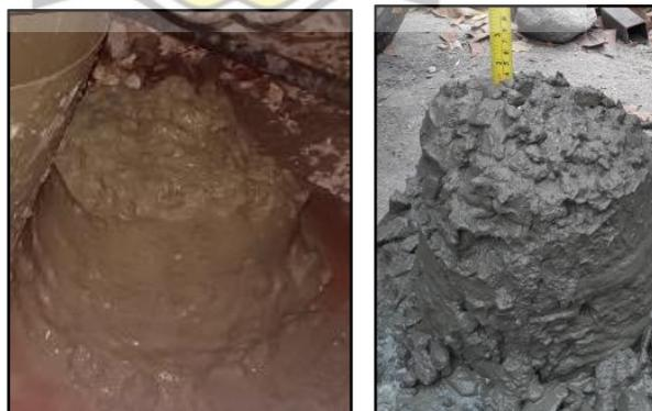
Gambar 3.61 Uji Slump Test Beton Ready Mix
