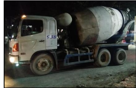
Gambar 3.37 Truck mixer concrete
