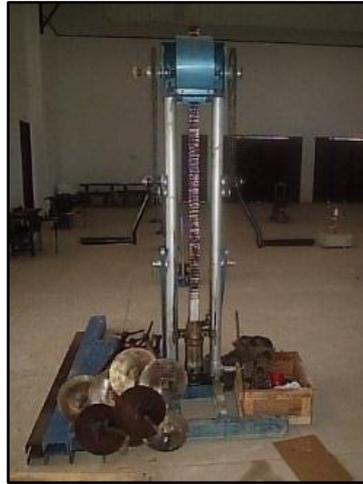
Gambar 3.8 Alat *Cone Penetration Test*
