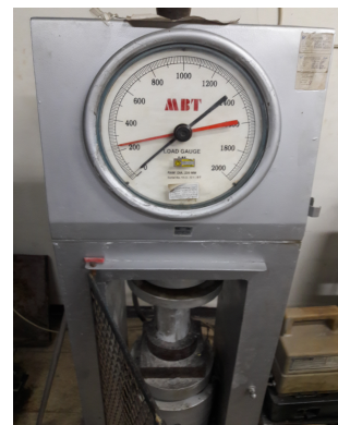
Fig. 1: Set-up of compressive strength test
