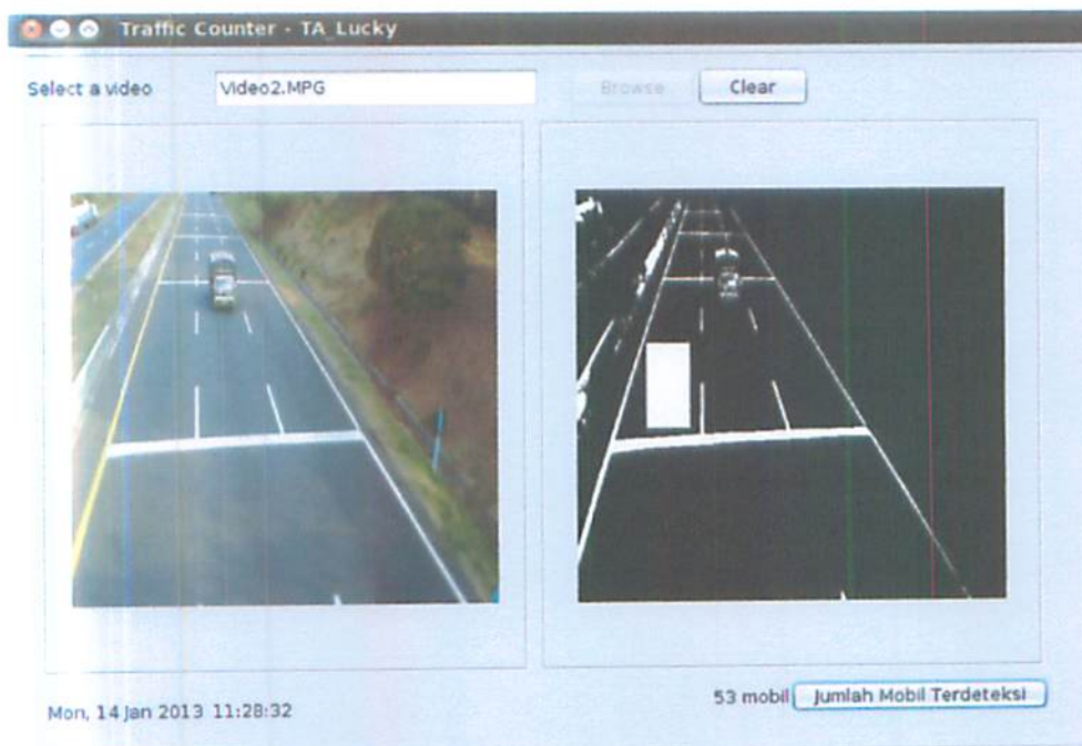
Figure 5.5 Application View The Result Of The Car Being Detected
