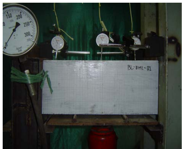
Figure 3. Experimental set-up with dial gauges and hydraulic jack loading equipment (Lelono and Widi, 2009; Susilorini, 2009a,b)
