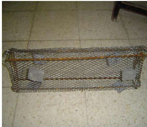
Figure 2. The placement of expanded metal sheet confinement for deep beams which cover the steel bar (Lelono and Widi, 2009; Susilorini, 2009a,b)
