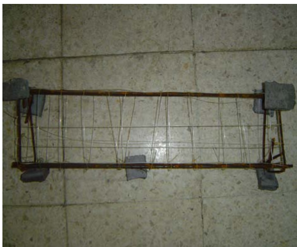
Figure 1. The placement of nylon mesh confinement for deep beams which cover the steel bar
