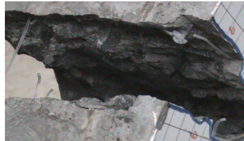
Figure 7. The broken nylon mesh is found mostly at the joint (Photograph by Setyanegara and Sagita, 2008)
