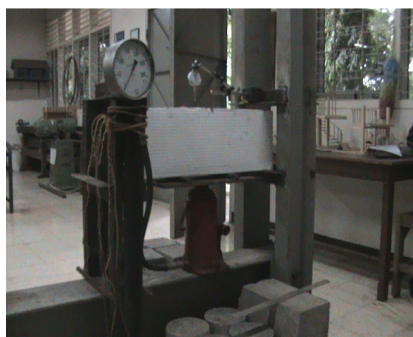
Figure 3. Third point flexural test (Photograph by Setyanegara and Sagita, 2008)
