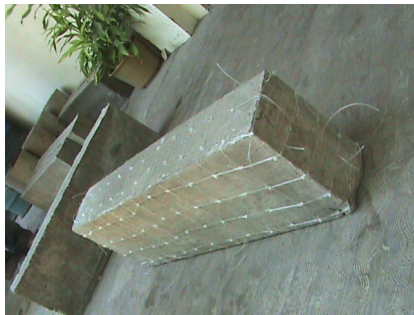
Figure 1. The confined beam specimen (Photograph by Setyanegara and Sagita, 2008)
