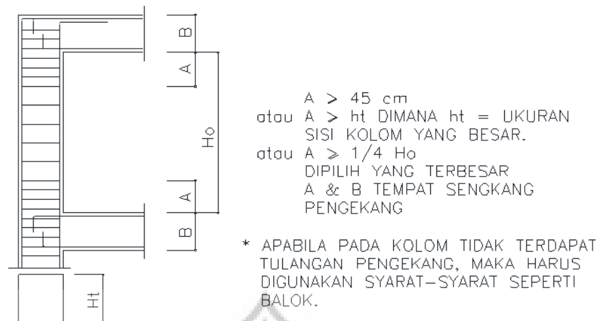
Gambar 4.12 Detail Jarak Sengkang Kolom
